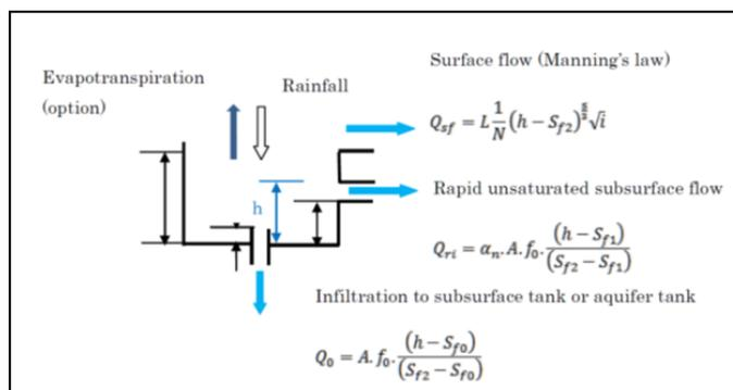
Figure 3: Schematic flow model level (IFAS System Instruction Guidebook, 2011:13)
