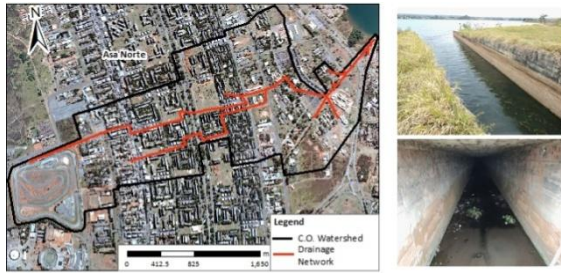
Figure 2. Drainage Network in the C.O. basin, outfall detail.
