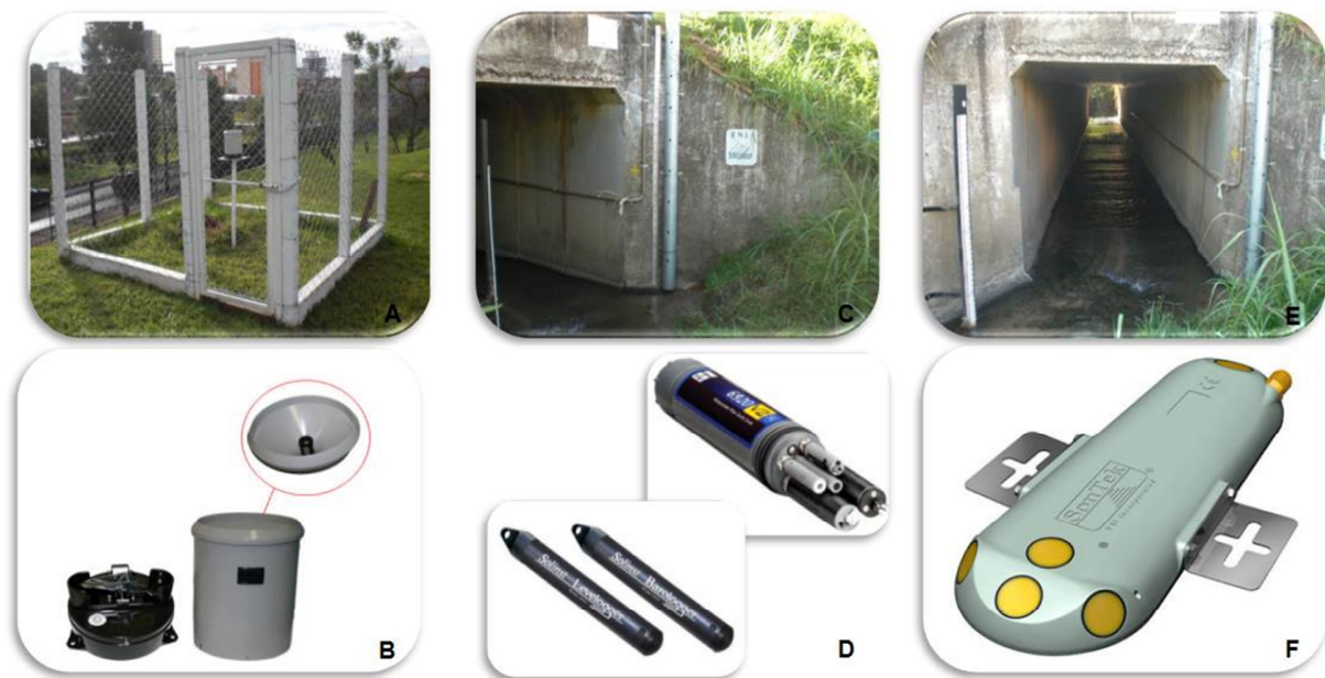
Figure 3 – Details of the network and its equipment:(A) protection fences for rain gauges; (B) tipping bucket rain gauge; (C) protection tube for the pressure transducer and multiparameter probe; (D) pressure transducer, barometer and multiparameter probe (above); (E) location of installation of the flowrate meter; (F) fixed ADCP type flow rate meter.
