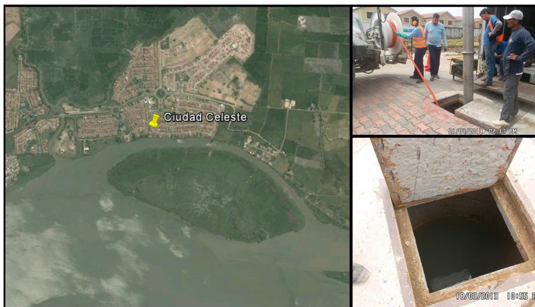
Figure 2. Islet location front of Ciudad Celeste community, we can also notice the storm drain chamber at it's full capacity due to the river flow; whereby, the Water Company services are hired, in order to use the hydrocleaner so the proper maintenance can be done.
