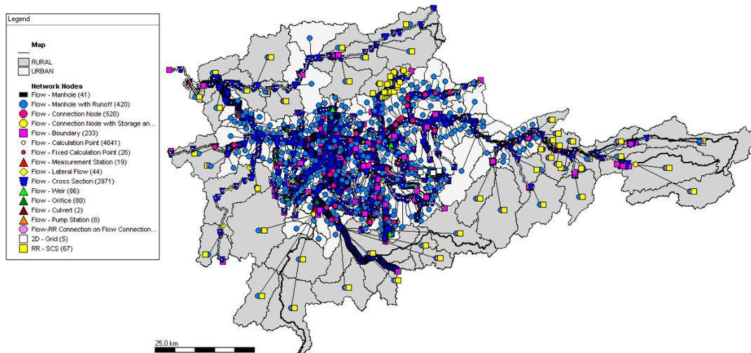
Figure 2: Complete schematization of UTB in SOBEK
