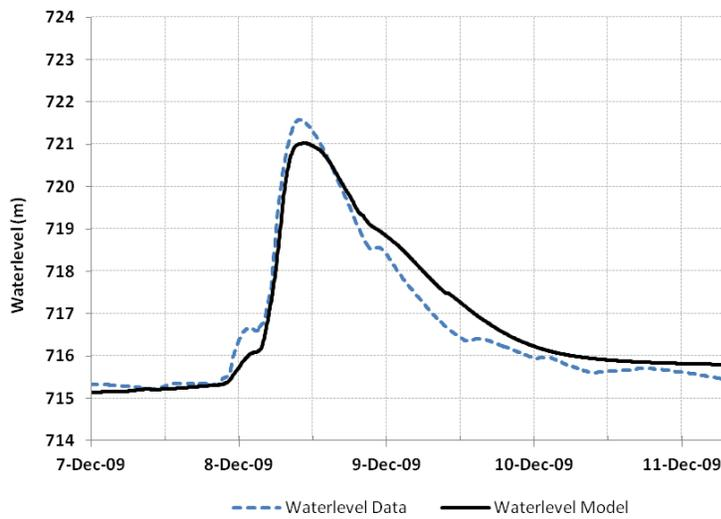
Figure 6: Comparison between water level calculated by the model and observed for the event of December 2009 - Ponte do Limão Station - Tietê River
