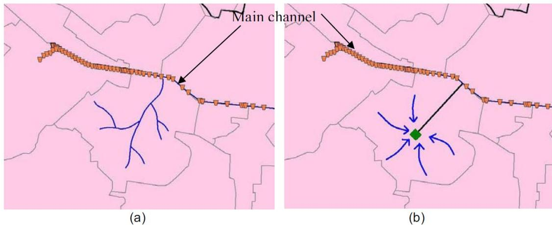
Figure 3: Drainage network in a sub-catchment conceptualized by a Manhole – Pipe system, extracted from Verwey *et al.* (2008)
