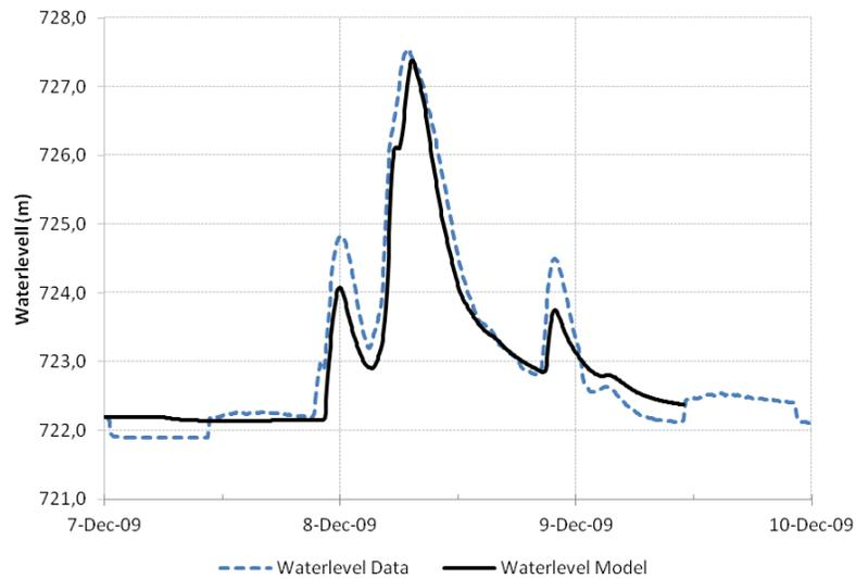
Figure 8: Comparison between waterlevel calculated by the model and observed for the event of December 2009 - Pacheco Chaves Station - Tamanduateí River
