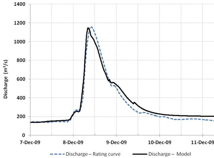
Figure 5: Comparison between discharge calculated by the model and observed (rating curve) for the event of December 2009 - Ponte do Limão Station - Tietê River
