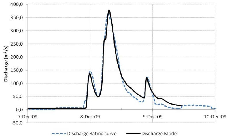
Figure 7: Comparison between discharge calculated by the model and observed (rating curve) for the event of December 2009 - Pacheco Chaves Station - Tamanduateí River
