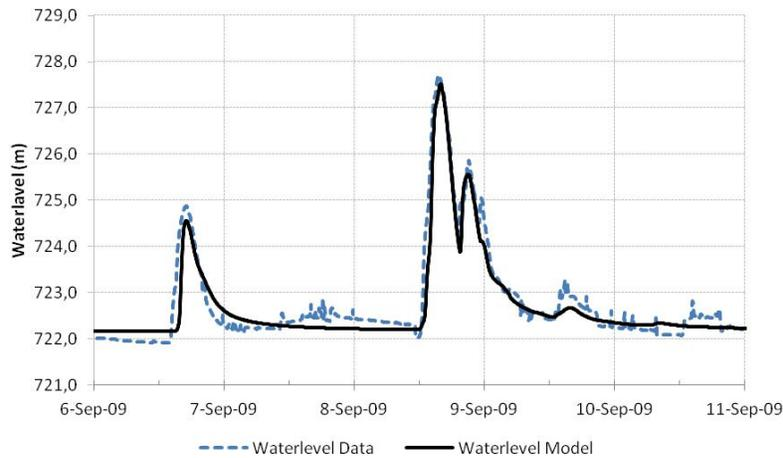
Figure 12: Comparison between waterlevel calculated by the model and observed for the event of September 2009 - Pacheco Chaves Station - Tamanduateí River
