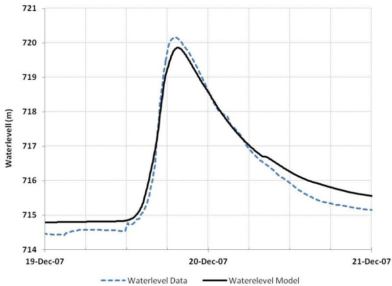
Figure 10: Comparison between waterlevel calculated by the model and observed for the event of December 2007 - Ponte do Limão Station - Tietê River
