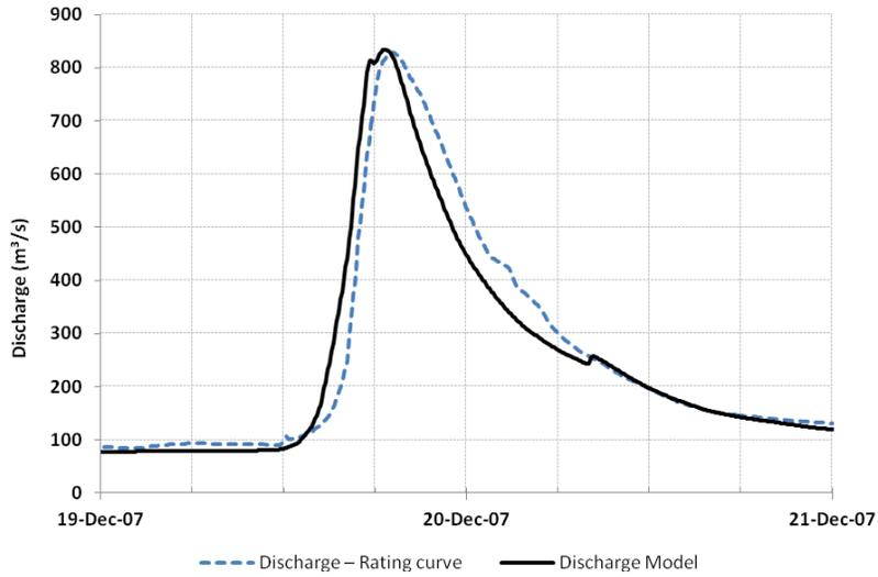
Figure 9: Comparison between discharge calculated by the model and observed (rating curve) for the event of December 2007 - Ponte do Limão Station - Tietê River
