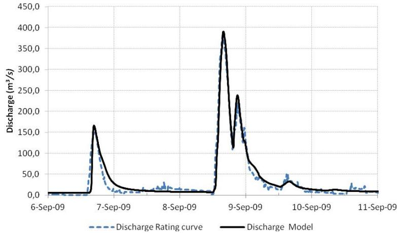
Figure 11: Comparison between discharge calculated by the model and observed (rating curve) for the event of September 2009 - Pacheco Chaves Station - Tamanduateí River
