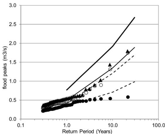
The Figure 2: QdF-rural and –urban models (lines). Flood peaks (dots) for CSOs (dark circles), natural flow (white circles) and total flow (dark triangles).
