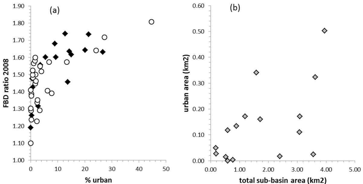
Figure 3: (a) Calculated 2008 FBD ratios at sub-basin outlets VS % urban for stream without bed incision (white dots) and observed active incision (black dots). (b) Urbanized sub-basin area VS total area for stream with incision only.
