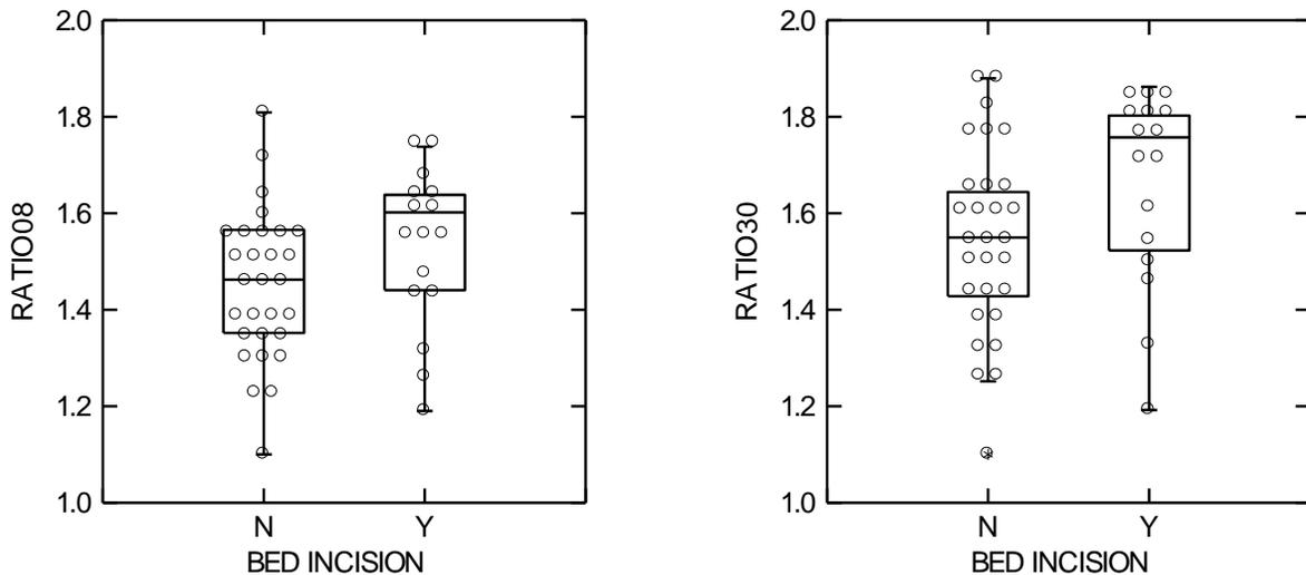
Figure 4 a, b: Box plot of calculated BFD ratios at sub-basin outlets respectively on 2008 (a) and (b) 2030. Two groups are considered: group 'Y' for incised stream bed and group 'N' for not incised stream bed. Boxes show quartiles 25%, 50%, 75% and lines bottom give 1.5 fold the inter range of upper and lower quartiles (stars indicate 3.0 folds inter range limits). Dots figure density distribution of data.
