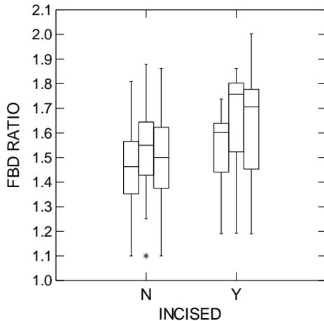
Figure 5: Box plot of calculated BFD ratios at sub-basin outlets. There are 3 boxes by group (Y and N) from left to right for 2008 managing runoff “as usual” and 2030 considering new rules for managing rainfall runoff. Two groups are considered: group ‘Y’ for incised stream bed and group ‘N’ for not incised stream bed. Boxes show quartiles 25%, 50%, 75% and lines bottom give 1.5 fold the inter range of upper and lower quartiles (stars indicate 3.0 folds inter range limits).
