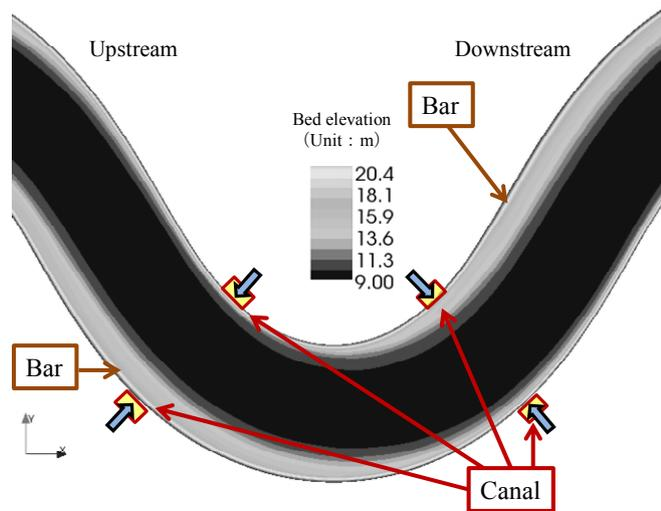
Figure 10: Bars in the meandering channel (Case 2-1)
