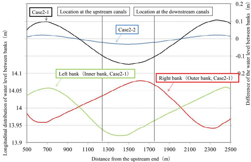
Figure 9: The longitudinal distribution of water level along both banks (Cases 2-1 and 2-2)
