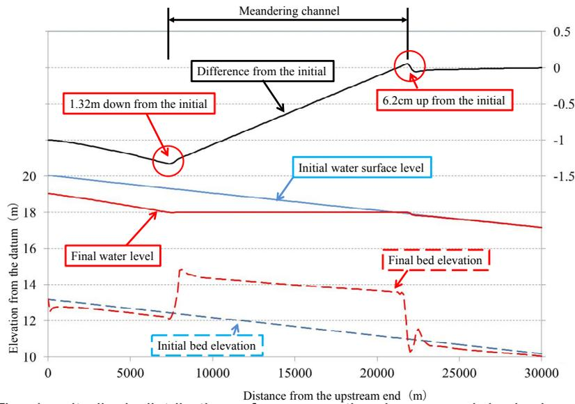
Figure 8: The longitudinal distribution of cross-sectional averaged bed elevation and the difference of cross-sectional averaged water depth from the initial value (Case 1)
