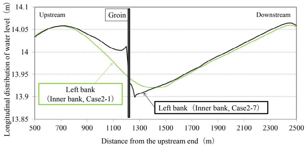
Figure 11: The longitudinal profile of water level along the inner bank (Cases 2-1 and 2-7)
