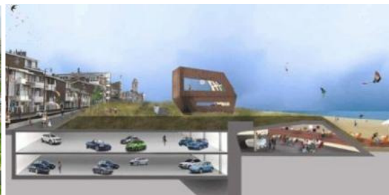
Figure 4b: Enforcement of the Katwijk coastal defence and dunes, in combination with the construction of an underground car park
