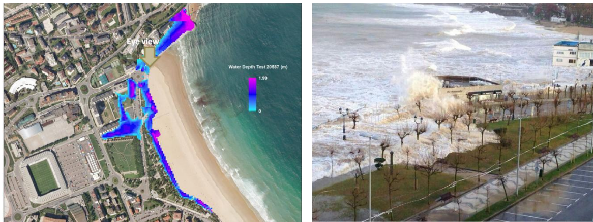
Figure 6 : (Left) Inundation extent and reached water depth (test 20587).(Right) Picture taken on March 1st, 2014 during an exceptional event.
