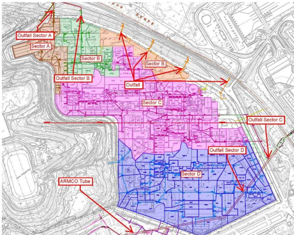
Figure 2: An example of Subbasin definition for Ascó NPP Esplanade
