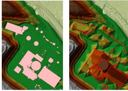
Figure 3. On the left, the DTM with building polygons. On the right the building footprint added to the TIN DTM, generating a DSM with noisy triangles
