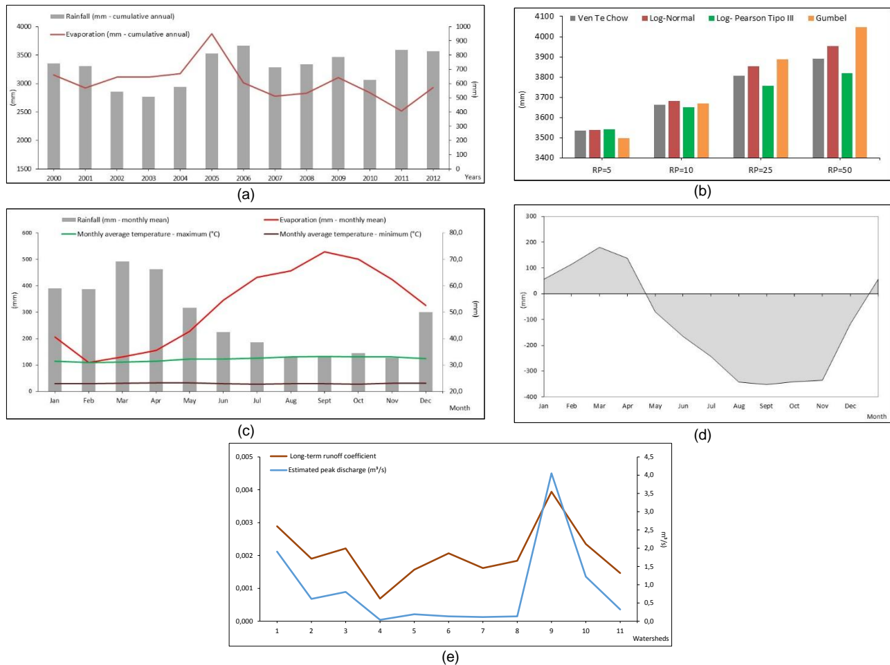
Figure 8: (a) Rainfall and evaporation by year; (b) Probability distribution functions and Return Period (RP); (c) Rainfall, temperature and evaporation by month; (d) Water balance in the study area; (e) Estimated peak discharge and runoff coefficient (ETR = Real evapotranspiration, P = Monthly average rainfall, EVP = evaporation, 1 - Água Preta, 2 - Bolonha, 3 - Tucunduba, 4 - 3 de Maio, 5 - Quintino Bocaiuva, 6 - Bernardo Sayão, 7 - Tamandaré, 8 - Doca de Souza Franco/Reduto, 9 - Una, 10 - Val-de-Cães, 11 - Mata Fome). Database (2000-2012) from National Institute of Meteorology (INMET).
